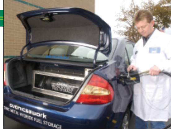
A tank with a metal hydride inside can hold three times more hydrogen than can be stored as a compressed gas in the same space.
